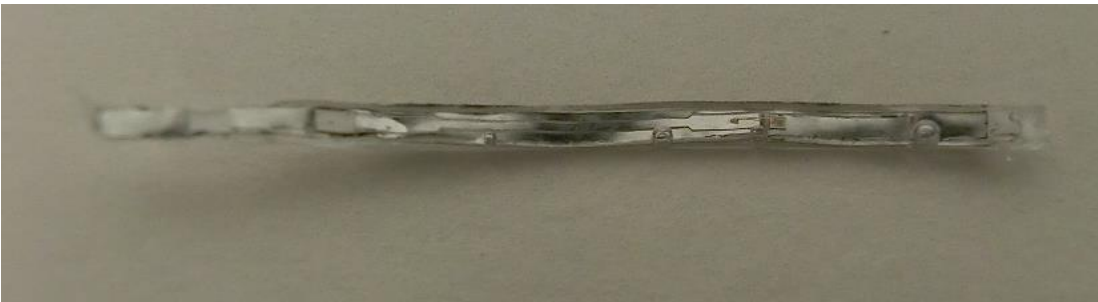
Flexible substrate made of silicone and platinum with a length of 22 mm and a width of ~1 mm.
