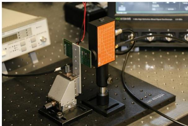
Figure 8: VCSEL driver test setup with driver board, photo receiver (orange) and high speed oscilloscope in the background.
