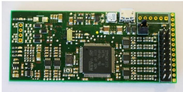
Figure 7: VCSEL driver PCB for system B with a size of 36 mm x 80 mm.
