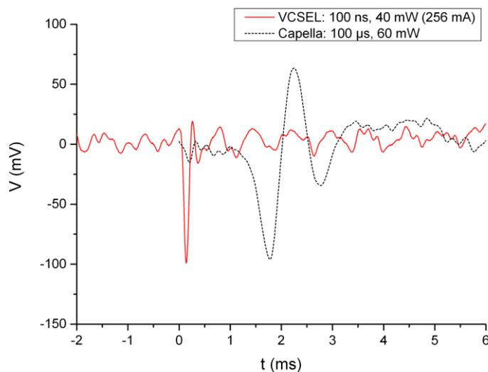
**Figure 10: Comparison of the artefact (in red) with an optically evoked CAP (in black), generated with the Capella laser system. In both measurements the laser pulse was applied at t = 0 and an amplification factor of 10000 was used.**
