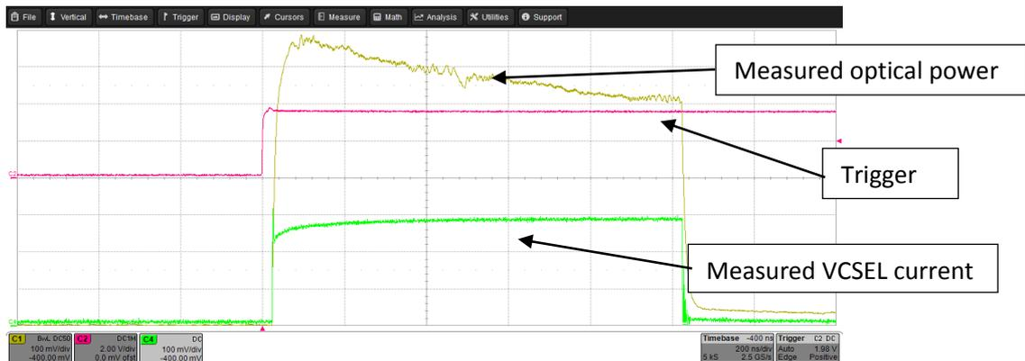
**Figure 9: Measured optical output power of the VCSEL for a 1000 ns pulse. Peak power is reached after  $\sim$ 50 ns and starts to decrease due to internal heating of the VCSEL and insufficient heat sinking.**
