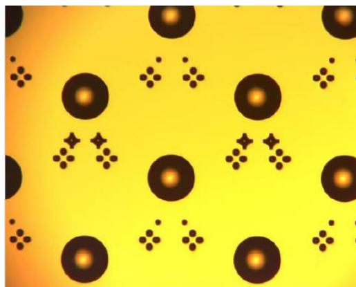
**Figure 3: Single micro-lens developed and fabricated by SUSS before dicing. The lens is 15  $\mu\text{m}$  high and the underlying slab has been polished down to 150  $\mu\text{m}$ .**
