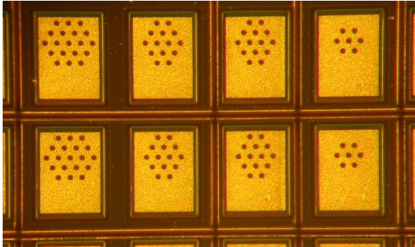
**Figure 2: Laser diced 1550 nm VCSEL arrays showing a hexagonal geometry with a 50  $\mu\text{m}$  pitch between apertures. The dicing lines are not in the centre of the dicing street but rather laterally offset toward some VCSELS to minimise the dicing boarder.**
