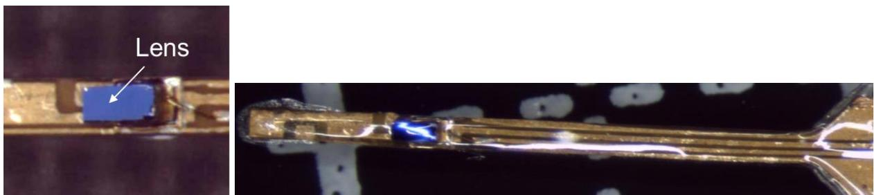
**Figure 5: Micrographs of System A++. Left: Close up of the VCSEL and the lens (blue) bonded to the polyimide substrate. Right: The tip of the substrate has a width of ~0.4 mm. After ~10 mm, it widens to provide better handling during tests.**
