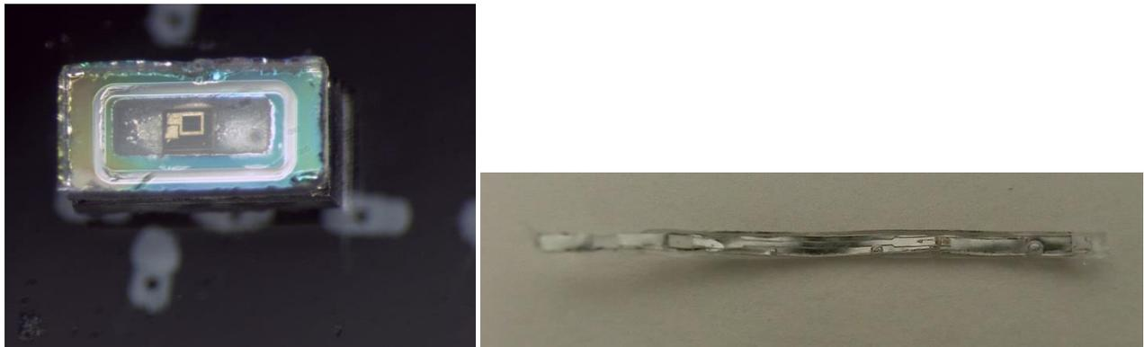
**Figure 4: Left: Hermetic package made from sapphire with a length of 1.5 mm and a width of 0.6 mm. The VCSEL can be seen in the cavity of the package. Right: Flexible substrate made of platinum and silicone. The device is 22 mm long and ~0.8 mm wide.**
