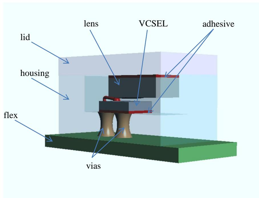
**Figure 1: Major components of the implantable laser source. The vias are electrical feedthroughs, which provide electric current to the VCSEL inside the hermetic package (i.e. housing and lid).**
