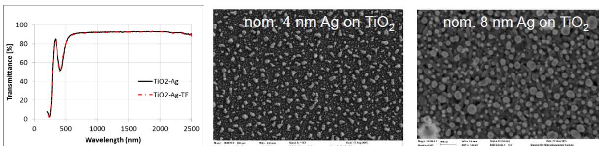
**Figure 6: The IR-Vis transmission spectra and SEM images of Ag coatings on borosilicate glass (TF = thiophenol).**
