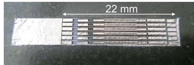
Figure 2: Array of substrate electrodes. Batch and automated processes are developed to manufacture new, reliable and flexible implantable substrates.
